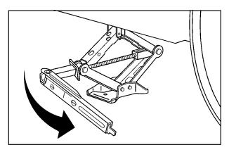
13. Lower the vehicle by turning the wrench counterclockwise. Lower the jack completely.
